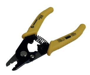
The Fiber Stripper is designed to strip the entire fiber. it can strip 1.6-3 mm fiber sheath up to 600-900 micron buffer coating. The second hole is designed to strip 900 micron buffer coating up to 250 micron coating. The third hole is used to peel off the 250 micron coating without leaving any nicks or scratches on the glass fibers.
