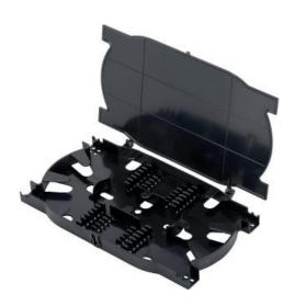
It is used for the termination and addition of fiber optic cables in order to preserve the cables that are fused inside fiber optic termination boxes. Each cassette has a capacity of 12 fiber terminations. In cases where further finishing is required, additional cassettes can be mounted on top of each other and side by side. Oct.
