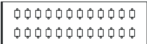
24 LC Duplex or 24 E2000 or 24 SC Simplex Vertical Adaptor Plate
